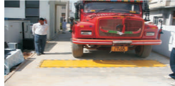
Check post Management system and WIM system
